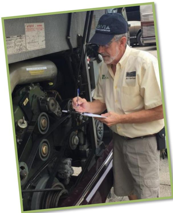
I felt the generator oil should be tested and he approved taking the sample. The report came back “critical”, requiring immediate repair. The report was provided to the client. Had the client purchased the RV without the oil sample and subsequent report there is a good possibility it would have failed on his way back to Reno.
